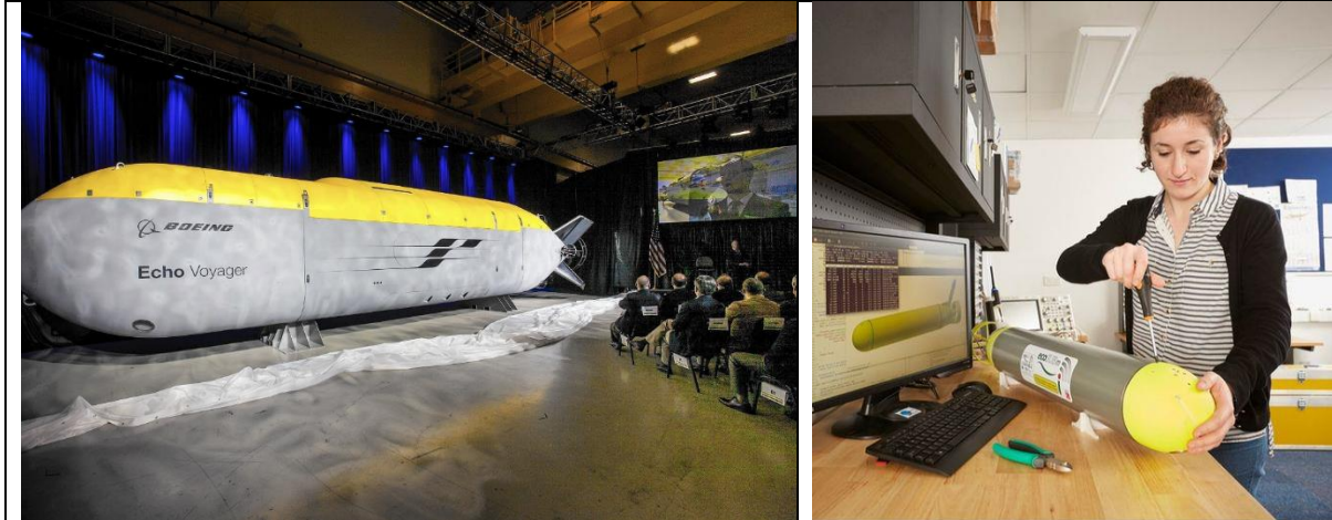
Figure 1. Left Boeing's Echo Voyager the basis for the US Navy XLUUVs. Right Planet Ocean's ecoSUB micro AUV.
