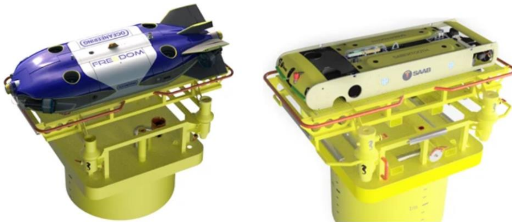
Figure 5. Blue Logic's Subsea docking station concept with a docked Freedom ROV (left) and a Saab Sabertooth (right).
