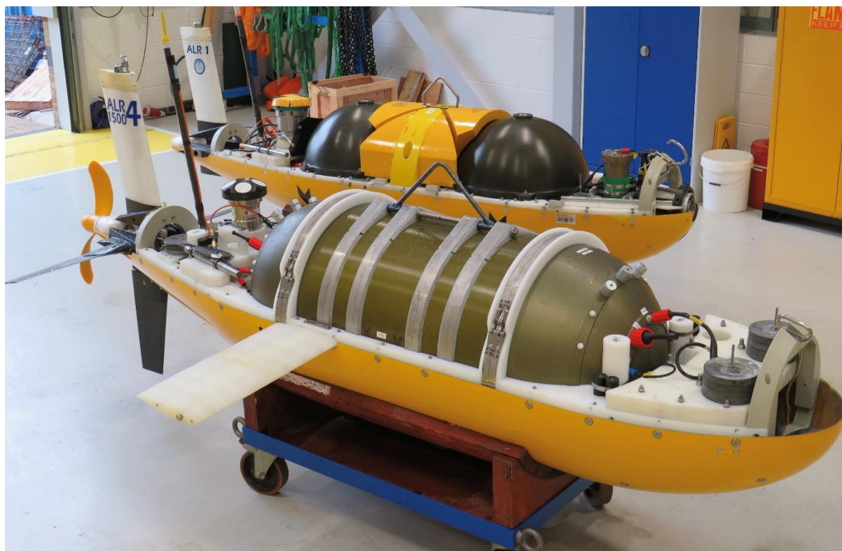
Figure 3 NOC's Autosub Long Range AUVs. ALR1500 foreground and ALR600 in the background
